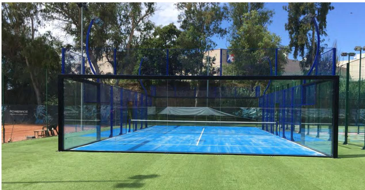
Toughened (or tempered) glass panels are used as the glass is specially treated so it will break into small blunt pieces under pressure making it much safer than shards of normal glass. The above photograph indicates a 'panoramic' padel court with framed end wall with no intermediate supporting steel posts.
